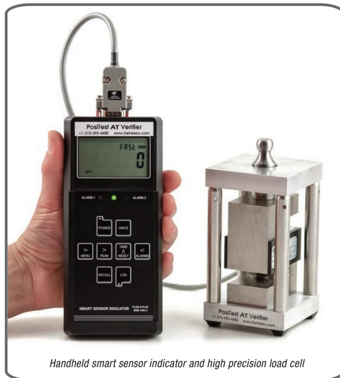
Handheld smart sensor indicator and high precision load cell
