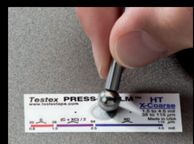
For use with OPTICAL Grade Testex™ Press-0-Film™ Replica Tape
