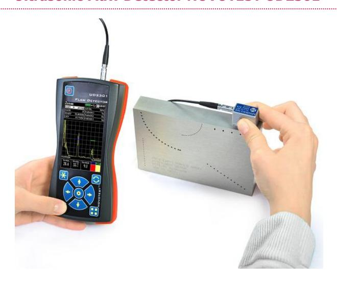
Ultrasonic flaw detector UD2301 is designed for nondestructive testing of metals, plastics, glass, composite materials, weld inspection and measurement of the thickness of the various products and structures.
